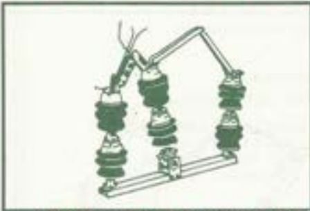
22 KV Double Stack Type Switch (Porcelain / Polymer)
